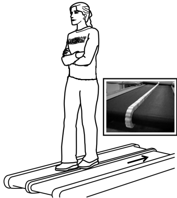
Fig. 1. A sketch of the experimental setup showing a subject walking on a treadmill-mounted balance beam. A picture of the balance-beam treadmill is also shown ( inset ).
