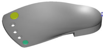
Figure 4 FO with adjustable metatarsal support elements. CAD model (left) and fabricated device (right). 2 nd to 4 th adjusters not shown in CAD model for clarity. Sections of the adjustable elements and their corresponding holes in the FO are threaded, allowing their height to be easily adjusted with a screwdriver.
