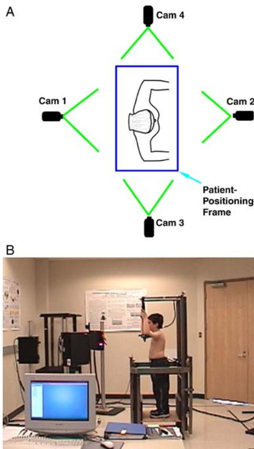
**Fig. 2** (A) Schematic layout of the InSpeck system arrangement composed of 4 digitizers, allowing for a 360° contour mapping of a subject's torso. (B) A patient-positioning frame is used to stabilize the patient during the data acquisition (typically 8 seconds per full trunk digitization).
