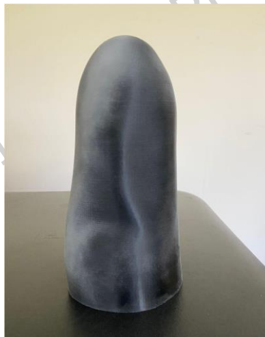
Figure 9. 3D-printed lower-limb cast surrogate
